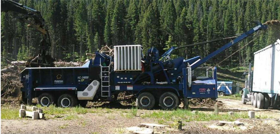
Figure 8. Broyeur Peterson Pacific 2400B
